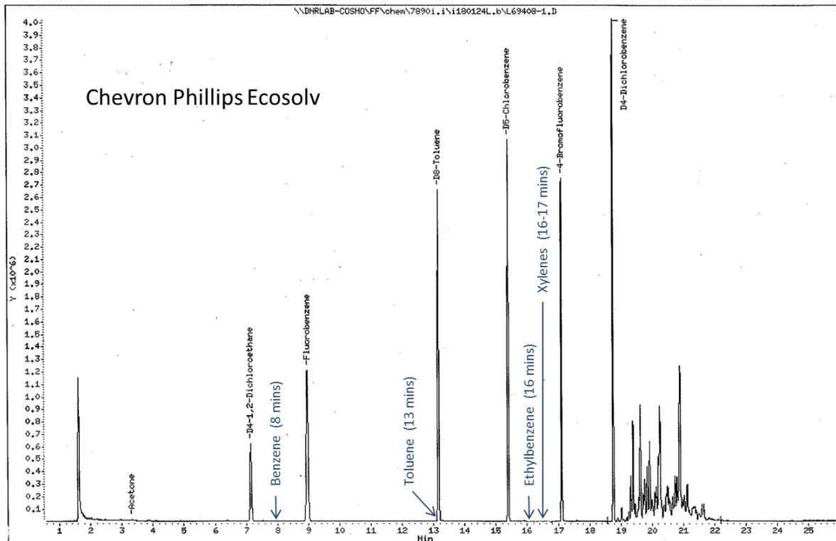
Figure 3. Chromatogram from GC/MS analysis of EcoSolv
